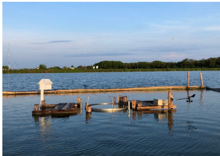
Figure 4 Setup of the Class-A evaporation pan over the LERD project oxidation pond.
